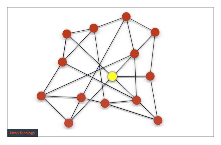
Mesh Topology is a type of network topology in which all devices in the network are interconnected. In a mesh topology, data can be transmitted by routing (sent the shortest distance) and flooding (sent to all devices).
