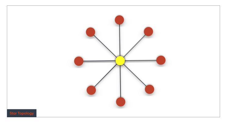
Star Topology is typically used when there is a single gateway that controls a number of nodes in the network. This topology is used in typical office Wi-Fi networks (gateway being the router) and also in LoRaWAN networks. A Star Topology has a number of pro's and con's:
